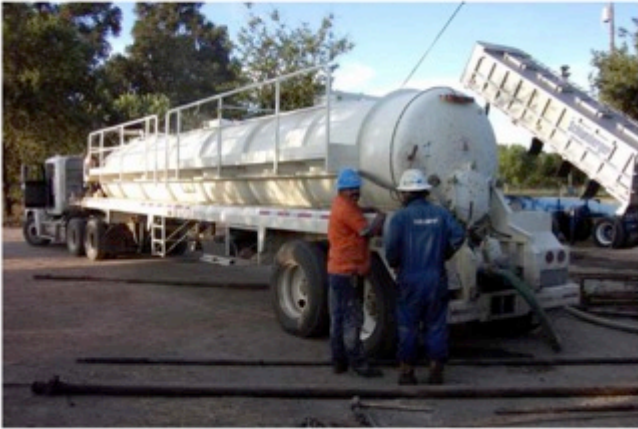
Pump Set (5000 psi, 7-10 bpm) Water Truck (150 – 300 gal. Used (typ).
