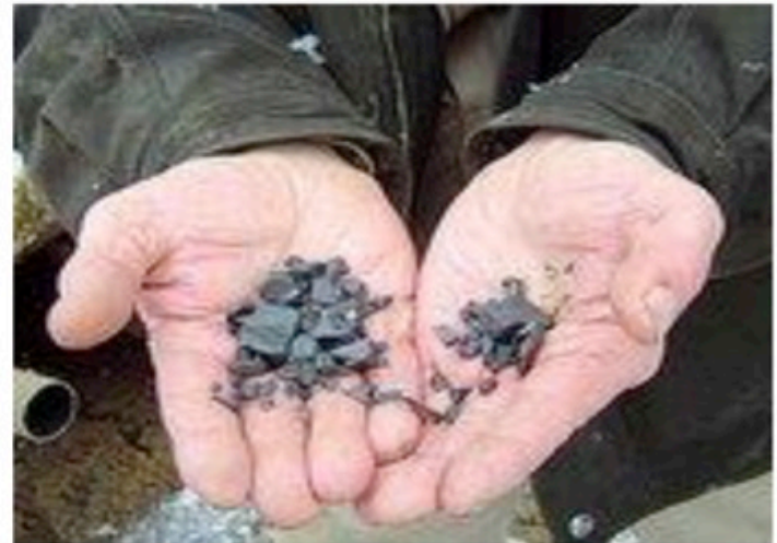
EcoSlice™ excavated rock and casing 11/16" – 3/4" (1mm – 18mm dia.)
